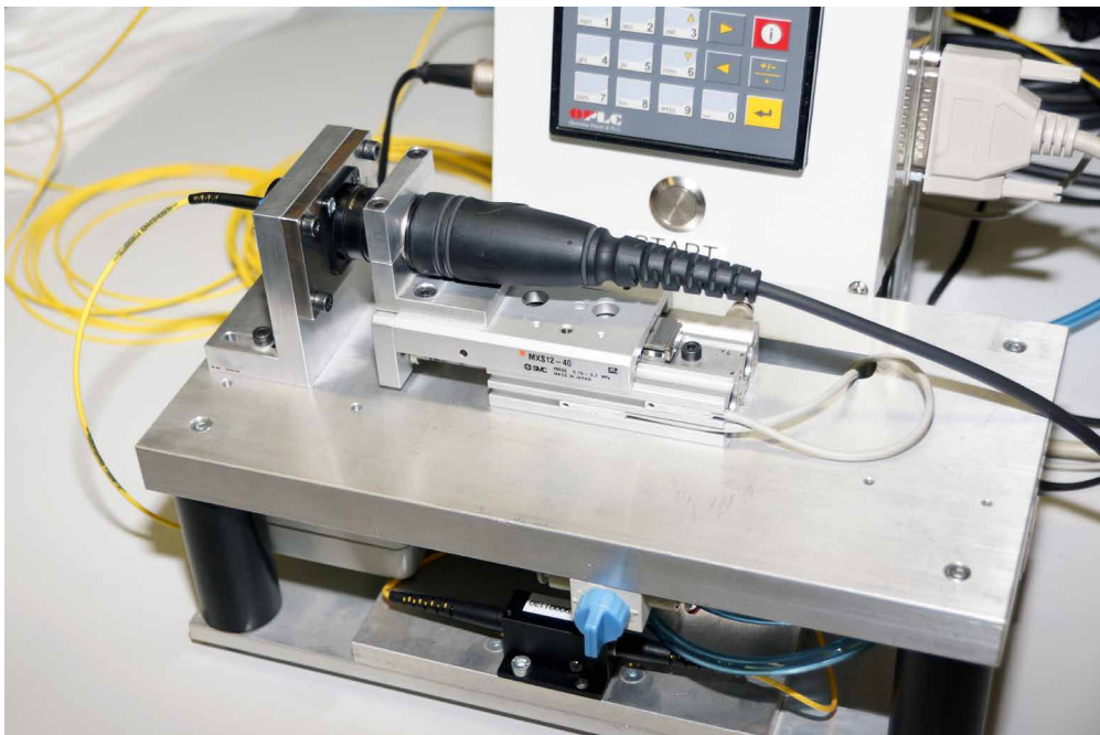
figure 7.b: fixture for 500 and 2.500 mating cycles
