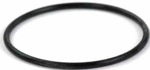
figure 9: O-ring after 2.500 mating cycles
