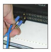
Alternatively the jack pairs may be pulled out by the use of two Bantam plugs (diagonally plugged in).
