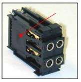
The two jack pairs have to be re-assembled in the right way so that the thicker body marked "left" is put on the left side with the mark outside and readable.
