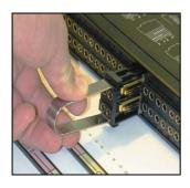
Pull one module out of the casing using the supplied disassembling pliers
