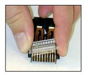
Finally snap on the cover (Insert it first at one side and then snap slightly into the opposite groove with a light pressure on the nose).
