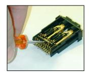
Pull out the configuration bars you need to exchange (preferably using a small screw-driver).
