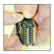
The two jack pairs are separated by spreading apart the rear parts to unlock the fixing mechanism till it is possible...
