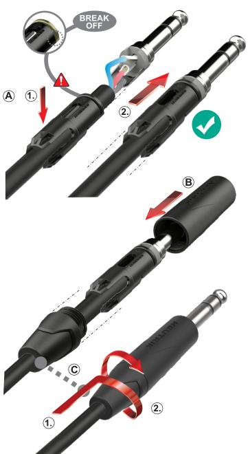
(A) Position the chuck onto the cable (1) and align chuck with plugfinger (2).
