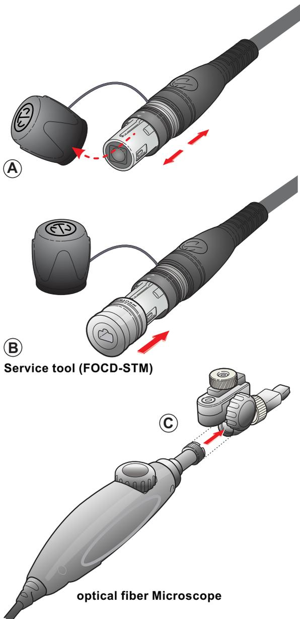
1. Disconnect both cable ends for safety reasons. Invisible laser radiation may be emitted from disconnected fibers or connectors. Do not stare into beams or view directly with optical instruments.
