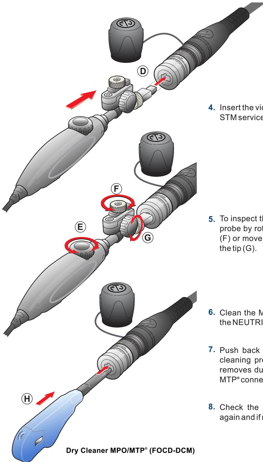
4. Insert the video probe tool into our NEUTRIK FOCD-STM service tool (D).
