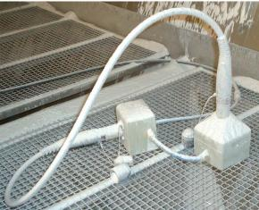
Table 12.b: Connected DRAGONFLY System before and after the dust chamber.
