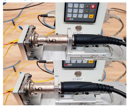
figure 7.b: fixture for 10.000 mating cycles
