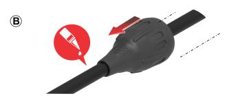
2 CABLE & BOOT ASSEMBLY WITH INSERTION TOOL
