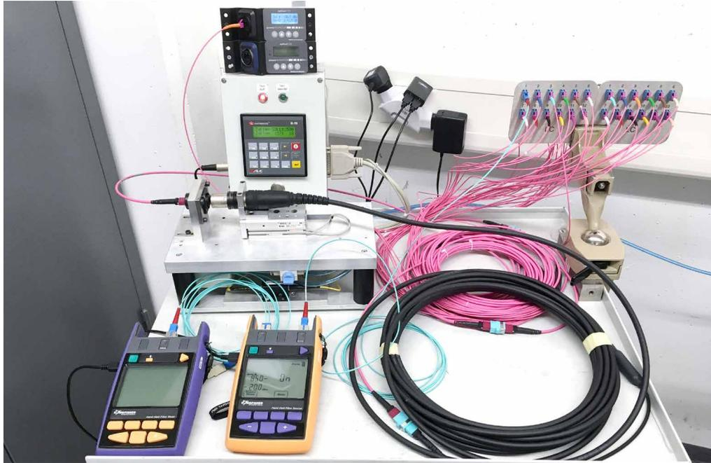
figure 6.a: measuring setup for lifetime test
