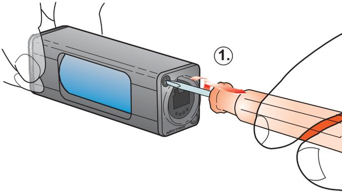
1. Untighten screws on both opticalCON chassis with a screw driver.
