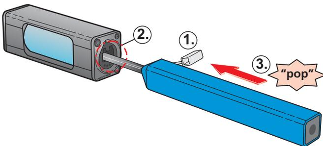
1. Remove dust cap. Insert the stick of the cleaning device.
