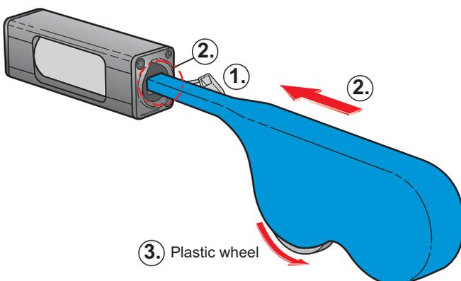
1. Remove dust cap and insert the tip of the dry cleaner.
