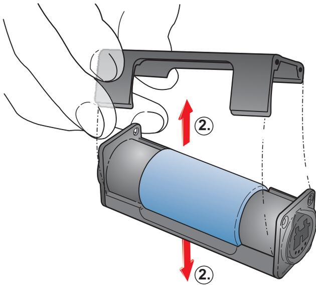
2. Remove top and bottom shelf of metal housing to release the protection tube.
